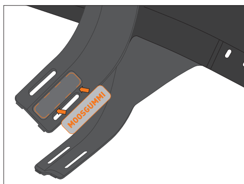
Adhere the sponge rubber to the mudguard (outer part).
